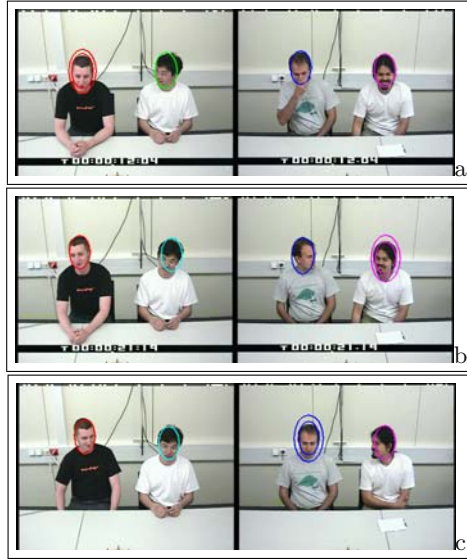
Fig. 3. Multi-object speaker tracker in the meeting room. The speaking status is inferred for each participant, a speaker is shown with a double ellipse
