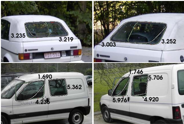
Fig. 8. Viewpoint invariance. Note that the bottom-right image is affected by projective errors, thus the rectangular window must be approximated by two ASEs
